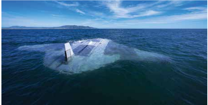
HFSWRs are fixed-site installations located right at the shoreline. From a countermeasures perspective, USVs and UUVs, such as the Manta Ray (above) developed by DARPA and Northrop Grumman, can maneuver very close to the victim radar and activate their jamming payloads. | NORTHROP GRUMMAN IMAGE
